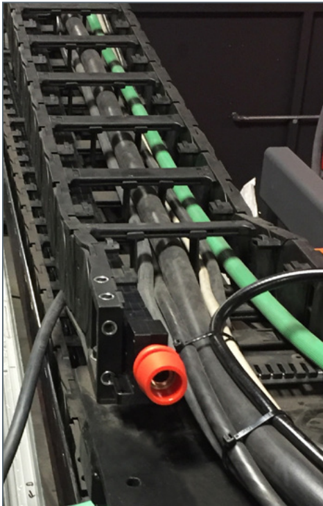
Guide Module® FLEX system installed on igus® e-chain® cable carriers in a traversing robotic application.
